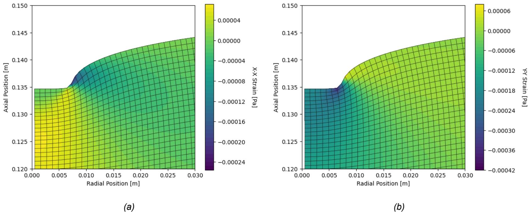
Figure 2. Strain for 150 element mesh with no slip condition on showing X-X (a) and Y-Y (b) strain fields zoomed into the top left area where the punch is acting. Full images are shown in appendix 6.1 (Appendix 6.1).
