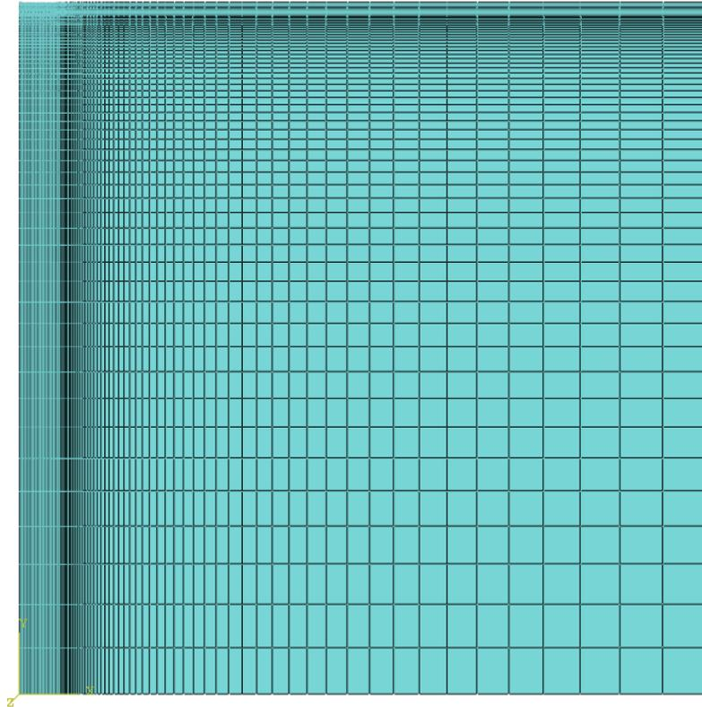
*Figure 5. Refined mesh biased toward the punch location (top left).*
