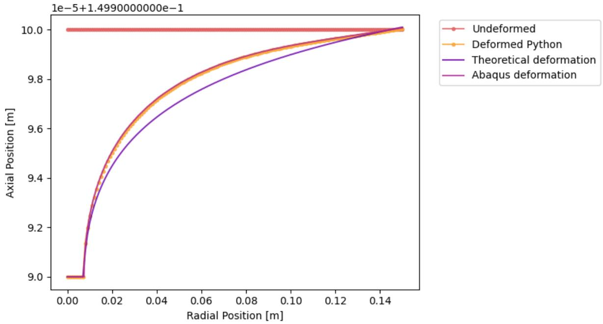
Figure 8. Full field view of the deformed shape of the Python based FEM analysis. Overlaid on the plot are the two validation method curves for the deformation of the top of the sample surface. All plotted deformations have the same scale factor applied.
