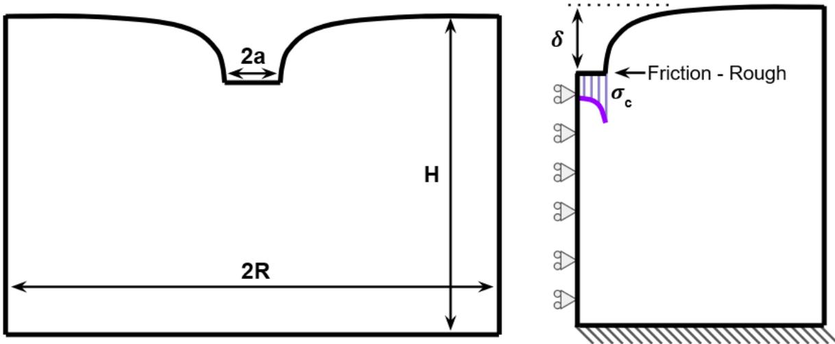
Figure 1. Overall sample geometry as well as symmetric geometry used for this analysis.
