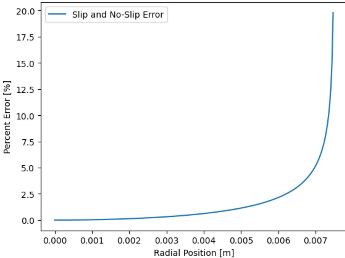
Figure 6. Percent error between slip and no slip theory equations for Y-Y stress.
