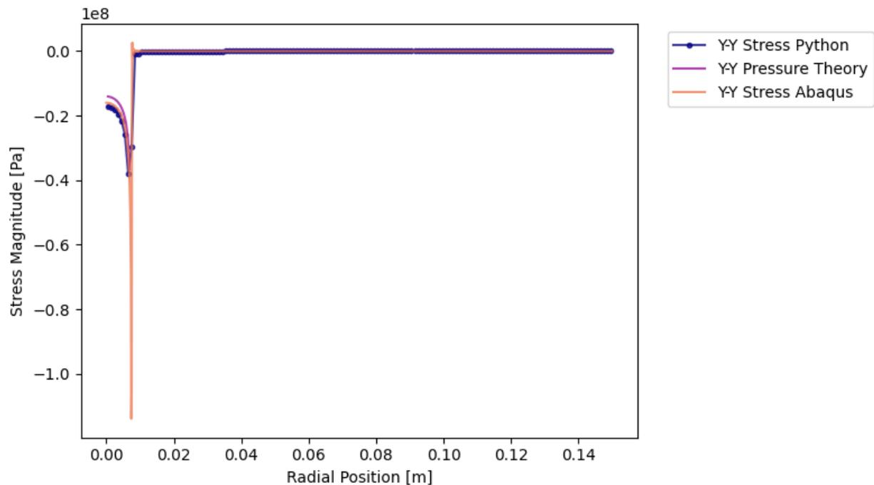
Figure 7. Comparison of the Y-Y stress distribution along the top elements for the Python based FEM analysis as well as the two validation methods.
