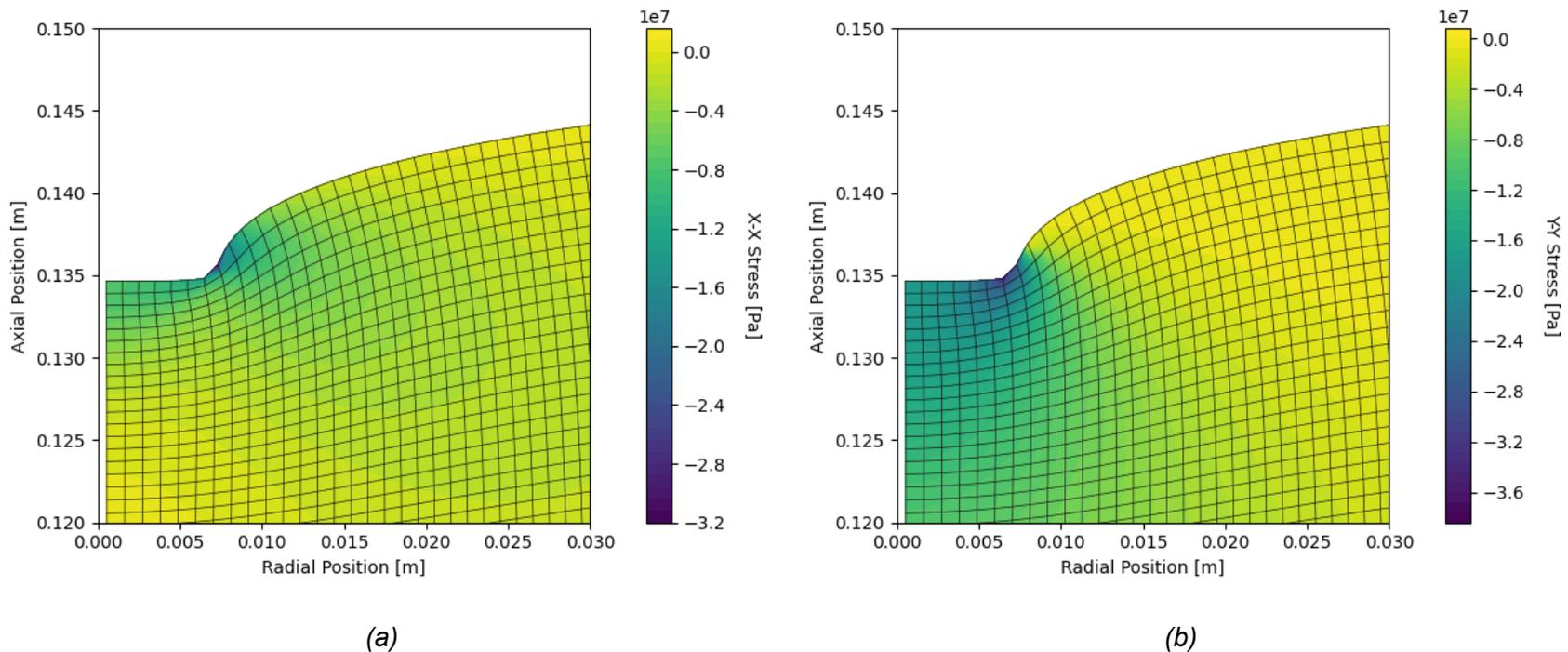
Figure 3. Stress for 150 element mesh with no slip condition on showing X-X (a) and Y-Y (b) stress fields zoomed into the top left area where the punch is acting. Full images are shown in appendix 6.1 (Appendix 6.1).
